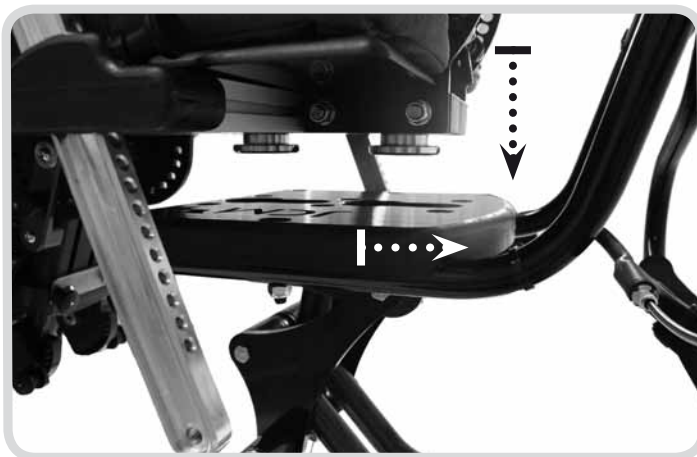
View from the side showing the seating unit lugs lowering into the interface plate cut outs.
